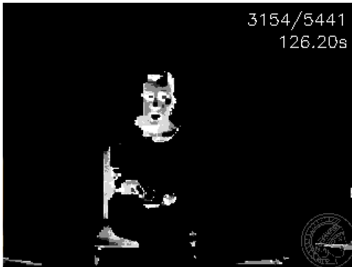
Figure 4: A screen shot of a video showing detected skin regions. Very white regions correspond to high probabilities for skin regions. The chair is also part of the skin-region as it has almost the same color as the gesturer. See figure 3
