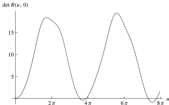
FIG. 5.  $\det \mathbf{B}(u, 0)$  for a plane wave spacetime with  $\mathbf{H}(u)$  given by (3.95) and  $h = 2/3$ . The zeroes correspond to locations of conjugate hyperplanes. They occur in closely-spaced pairs separated by approximately  $3.8\pi$ . Note that  $\mathbf{H}(u)$  has the shorter period  $2\pi$ .
