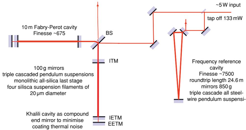
**Figure 2.** The basic optical layout for the first round of experiments in the AEI 10 m prototype facility. The frequency reference cavity and the main interferometer along with the most relevant design parameters are shown. Note that only 5 W input power will be used for the first experiments.
