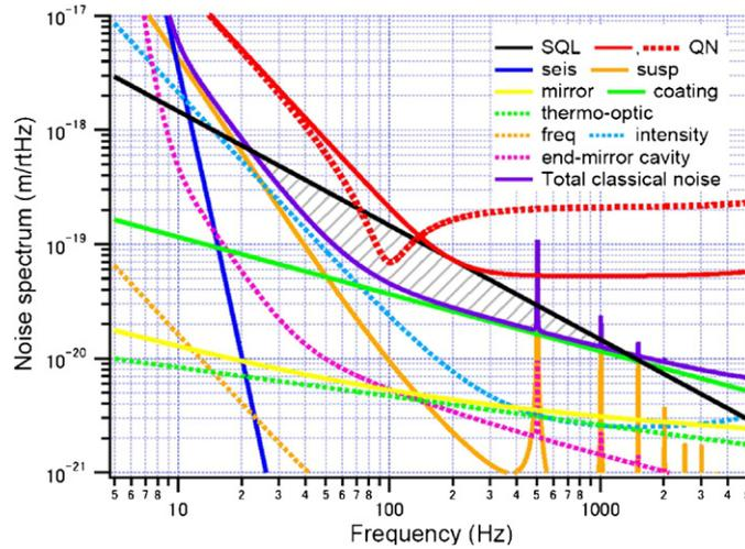
**Figure 3.** The design sensitivity of the AEI 10 m prototype interferometer. The black straight line is the SQL, the red solid curve is the sum of quantum noise, the blue solid line is the sum of all classical noise sources. The dashed area inbetween the sum of classical noise and the SQL is the QND regime that we hope to be able to explore by applying e.g. the back-action evasion technique (red dashed curve).
