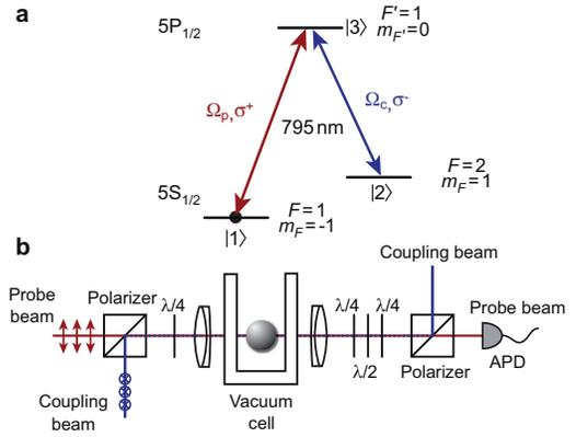
FIG. 1: (a) EIT  $\Lambda$ -system in <sup>87</sup>Rb ( $D_1$ -line). The transition between the two ground states  $|1\rangle$  and  $|2\rangle$  is insensitive to magnetic field fluctuations to first order at  $B \simeq 3.23$  G. (b) Experimental setup. Probe and coupling beam are used in a collinear configuration and are focussed onto the atoms in the optical lattice.
