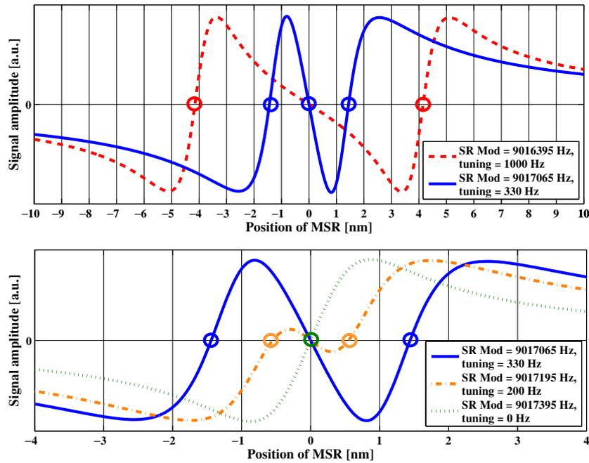
**Figure 3.** Signal recycling error signals derived from an RF modulation demodulation technique versus microscopic position of the signal recycling. The error point is plotted for various modulation frequencies corresponding to detunings of the signal recycling cavity between 1000 Hz and 0 Hz. By increasing the modulation frequency the structure gets more and more squeezed.
