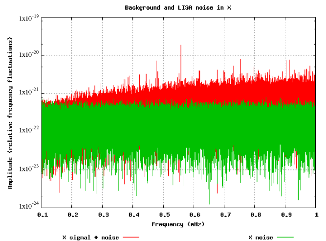
FIG. 8 (color online). The amplitude of the Fourier transform of the WD-WD galactic background gravitational wave signal and of the LISA instrumental noise entering into the TDI combination X .
