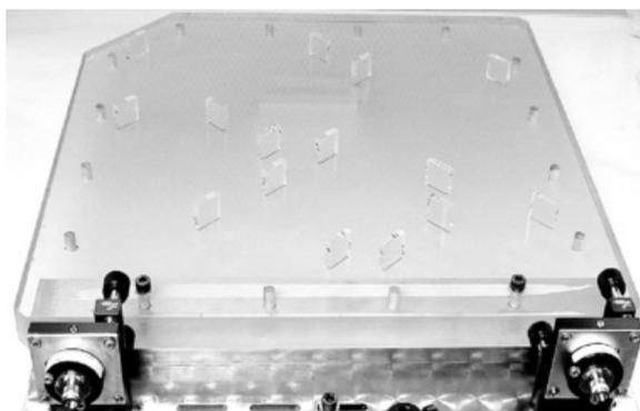
**Figure 5.** Prototype optical bench fabricated using hydroxide-catalysis bonding.
