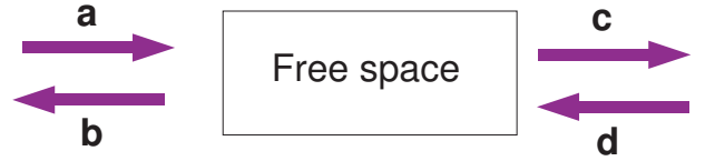
FIG. 2: The fields entering and exiting a region of free space are shown. Propagation operators are characterized by the propagation distance (and orientation relative to the source polarization, in the case of the GW signal).
