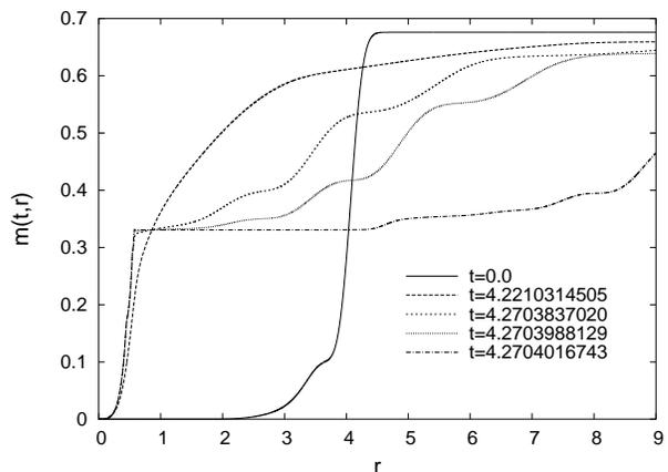
FIG. 1: Formation of a black hole for highly supercritical initial data. We plot the mass function  $m(t, r)$  at the initial time and at four late times. The total mass (measured in units  $3\pi/8G$ ) is 0.67 (see the plateau of the initial profile). During the evolution the function  $m(t, r)$  develops a second inner plateau which indicates formation of the Schwarzschild black hole with mass  $M_{BH} = 0.33$ .
