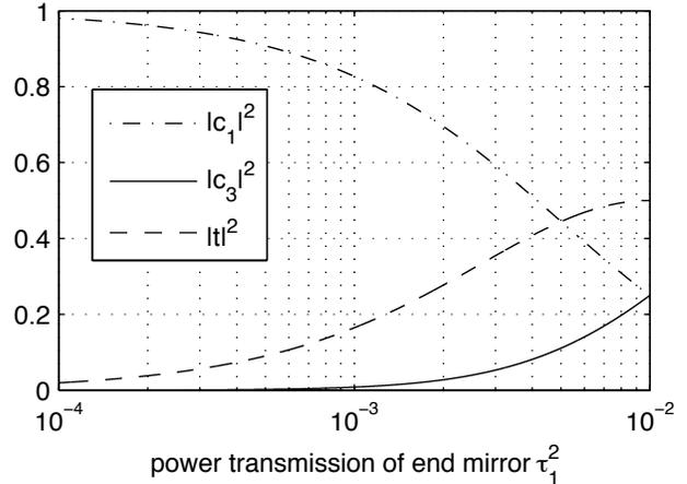
Fig. 4. Powers of the two reflected ports and the transmitting port as a function of end mirror transmittance  $\tau_1^2$  for a coupler with  $\rho_0^2 = 0.99$  and  $\eta_2 = \eta_{2,\min}$  for a tuning of  $\phi = 0$ .
