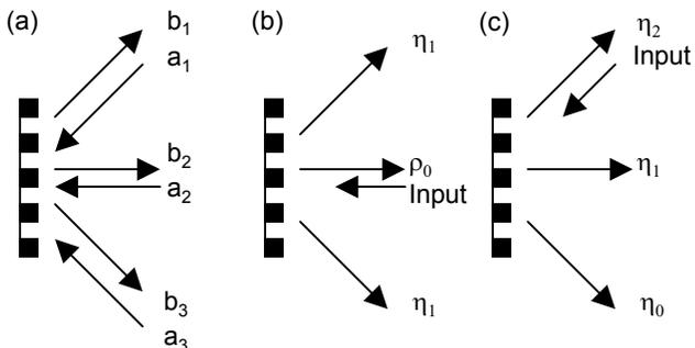
Fig. 1. A 3-port reflection grating: (a) labelling of the input and output ports, (b) amplitudes of reflection coefficients for normal incidence, (c) for 2nd order Littrow incidence.
