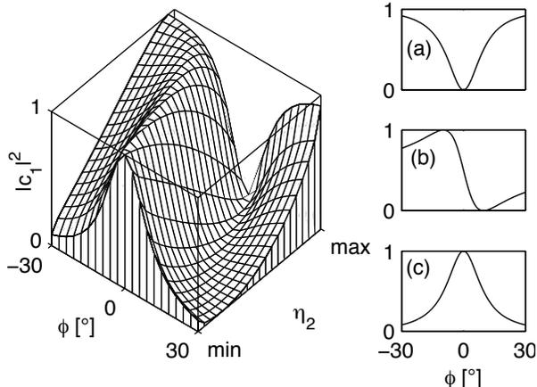
Fig. 3. Power  $|c_1|^2$  of cavity back reflecting port for gratings of different values of  $\eta_2$ . Left: Power as a function of  $\phi$  and  $\eta_2$ . Right: Power as a function of  $\phi$  for (a)  $\eta_2 = \eta_{2,\max}$ ; (b)  $\eta_2 = [(\eta_{2,\max}^2 + \eta_{2,\min}^2)/2]^{1/2}$ ; (c)  $\eta_2 = \eta_{2,\min}$ . Cavity parameters:  $\rho_0^2 = 0.5$ ,  $\rho_1 = 1$ .
