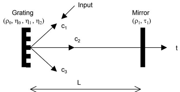
Fig. 2. A Fabry-Perot cavity with a 3-port grating coupler and a conventional end mirror. The amplitudes of the fields of interest ( $c_1, c_2, c_3, t$ ) are indicated by arrows.
