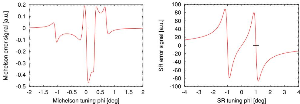
**Figure 6.** Computed error signals for the Michelson (left) and SR mirror (right) for a detuned operating point ( $T_{\text{SR}} = 1\%$ , detuning  $1^\circ$ ,  $f_{\text{det}} = 690$  Hz).
