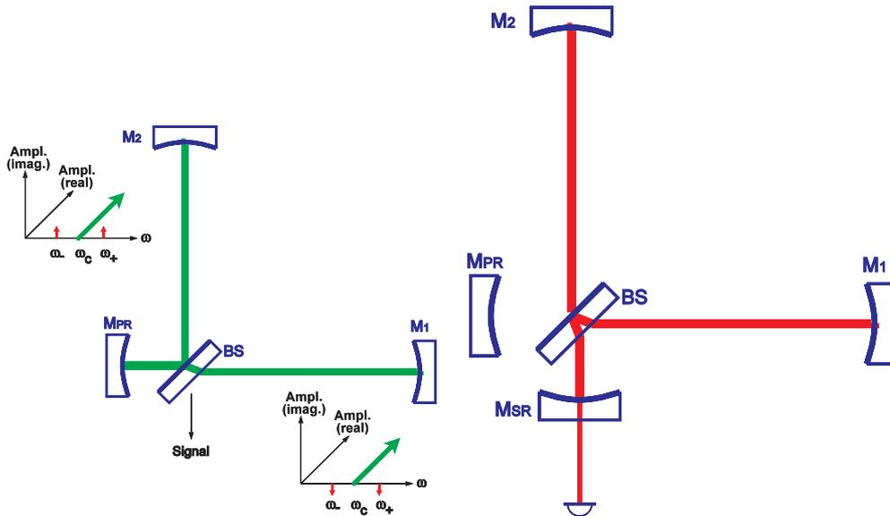
**Figure 2.** Left image: a gravitational wave produces phase modulation sidebands of opposite sign in the two arms. They are separated from the carrier by the beamsplitter. Right image: the signal sidebands can be resonantly enhanced in the signal recycling cavity, thus increasing the signal storage time.
