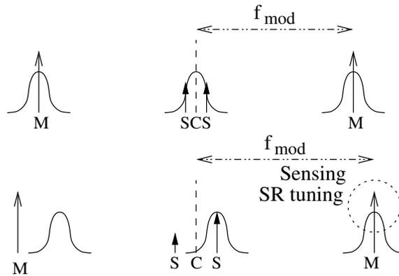
**Figure 5.** Schematic diagram of the SR cavity resonances for broadband (top) and detuned (bottom) signal recycling.  $C$  is the carrier frequency,  $S$  are the signal sidebands and  $M$  the Schnupp modulation sidebands.
