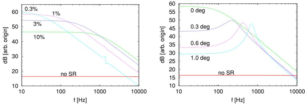
**Figure 4.** Transfer function of GEO 600 for gravitation wave signals for different power transmissions of the signal recycling mirror in broadband mode (left), and for different tunings with a 1% mirror in detuned mode (right).
