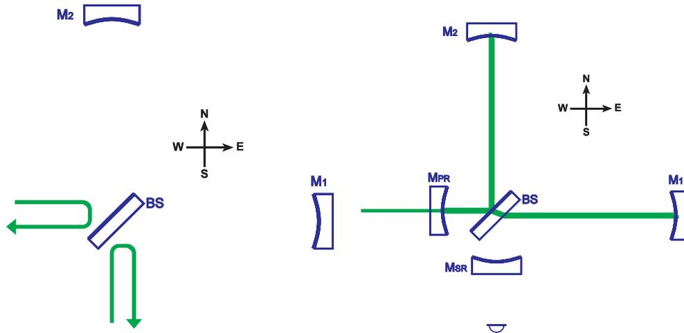
**Figure 1.** Left image: a Michelson interferometer in the dark fringe condition will essentially look like a mirror from both ports. Right image: power recycling resonantly enhances the light power circulating in the arms.
