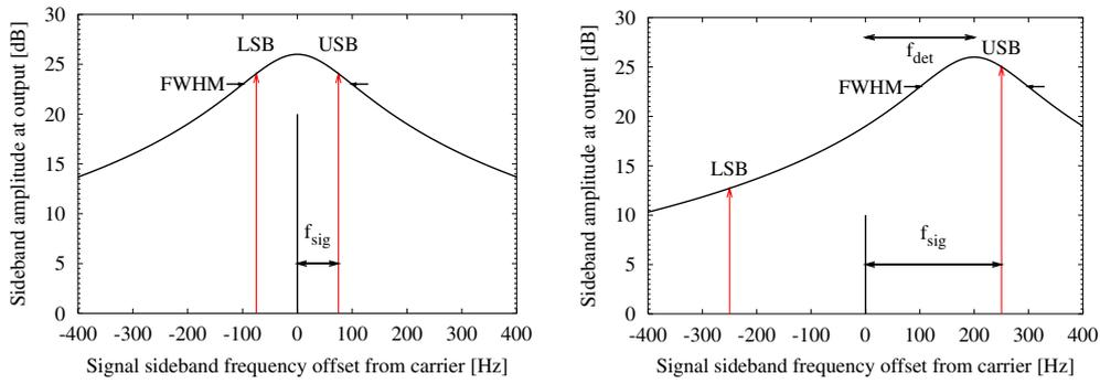
**Figure 3.** Schematic diagram of the SR cavity resonance for broadband (left) and detuned (right) signal recycling. LSB and USB are the signal sidebands for a gravitational wave of frequency  $f_{\text{sig}}$ .
