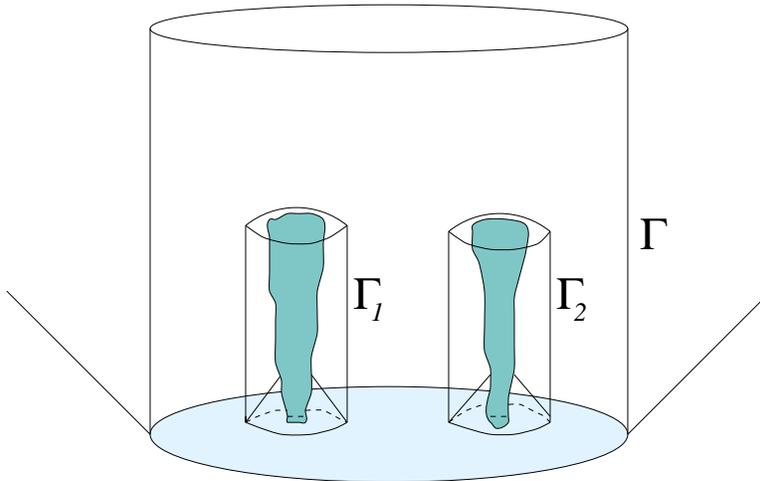
Figure 10: *CCM for binary black holes, portrayed in a co-rotating frame. The Cauchy evolution is matched across two inner worldtubes  $\Gamma_1$  and  $\Gamma_2$  to two ingoing null evolutions whose inner boundaries excise the individual black holes. The outer Cauchy boundary is matched across the worldtube  $\Gamma$  to an outgoing null evolution extending to  $\mathcal{I}^+$ .*
