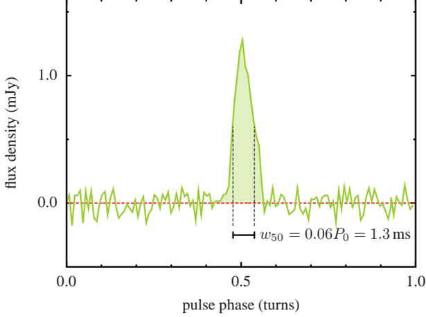
**Figure 1.** Folded pulse profile of PSR J1952+2630 at 1.4 GHz from the 576 s follow-up observation on 2010 September 20. The resulting period-averaged flux density is  $70 \mu\text{Jy} \leq S_{1400} \leq 100 \mu\text{Jy}$  (depending on the precise pulsar position within the beam). The duty cycle is 6% of the pulsar period  $P_0$ . The dispersive delay across a frequency channel is 0.3 ms.
