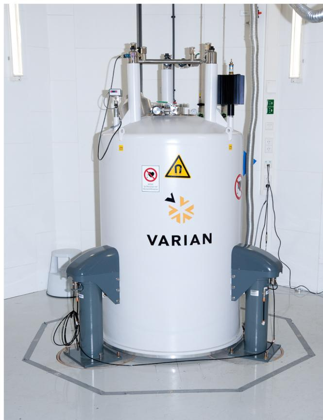
**Figure C.1:** 7-T superconducting magnet inside the PENTATRAP laboratory.
