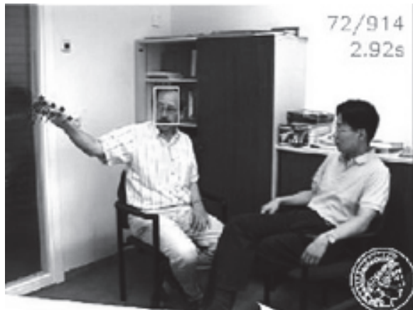
A screen shot of a video with moving corners shown in blue. The rectangle is the region selected by the user as a model for the skin color (white)
