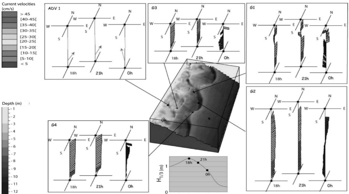
Figure 2. Hydrodynamic map of the current profiles over Leucate Beach bar system during the 22/01/2007 event, based on ADCPs measurements and ADVs.
