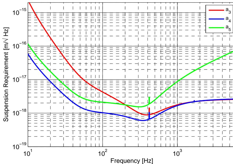
**Figure 5.** Suspension requirement for the maximum tolerable lateral grating displacement that is necessary to achieve the Advanced Virgo design sensitivity. The suspension required strongly depends on the readout port as well as the frequency of interest. At low frequencies the phase noise suppression in port  $a_3$  allows significant relaxation of the required suspension isolation. The narrow peak around 410 Hz is due to a resonance in the Advanced Virgo design, not a grating effect.
