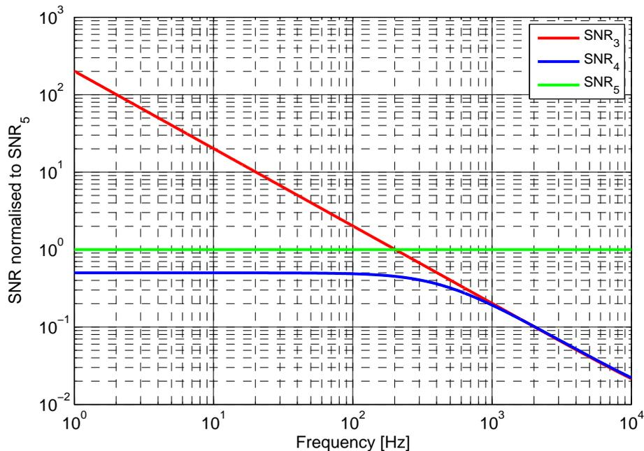
**Figure 4.** Signal to noise ratio of gravitational wave equivalent mirror displacement and lateral grating displacement at the three different output ports of a grating gravity. All traces are normalized to  $\text{SNR}_5$ .
