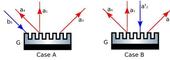
**Figure 3.** Input ( $b_0$ ,  $a'_2$ , shown blue) and output ( $a_1$ ,  $a_3$ ,  $a_4$ , shown red) light field amplitudes at a phase modulating grating in second-order Littrow-configuration in case A, and zeroth-order-Littrow configuration in case B (labels consistent with Figure 2).
