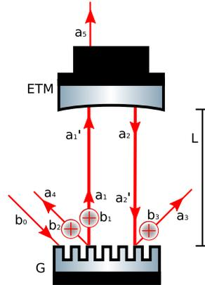
**Figure 2.** External input port  $b_0$ , internal input ports  $b_1$ ,  $b_2$ ,  $b_3$  (marked by encircled addition symbols) and the transfer ports  $a_1$ ,  $a_1'$ ,  $a_2$  and  $a_2'$  in a grating cavity
