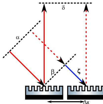
**Figure 1.** Wavefronts coupling through a diffraction grating. The wavefront (propagation vector shown in solid red) originates at  $\alpha$ , continues to  $\beta$  and is diffracted to  $\delta$ . Displacing the grating by a lateral distance of  $\Delta x$ , causes the wavefront (propagation vector shown red-dashed) to pass through the additional path length  $\zeta$  (propagation vector shown in solid blue).
