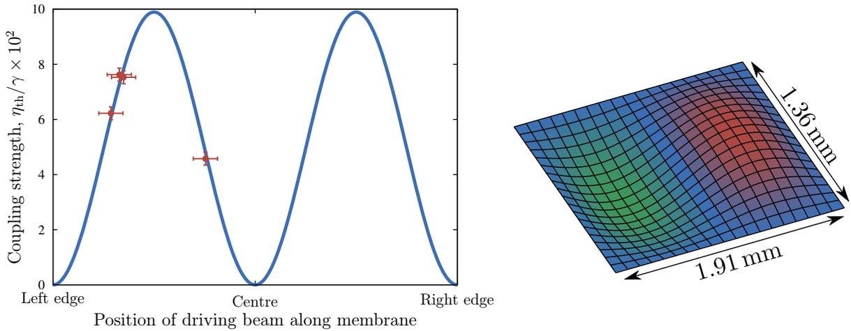
**Figure 4.** (a) The coupling parameters that fit the four datasets are consistent with the excitation of the (2, 1) mode of the membrane (shown in (b)); the solid curve represents the sinusoidal profile of the squared amplitude of this mode. (b) Vibrational profile of the (2, 1) mode of the membrane.
