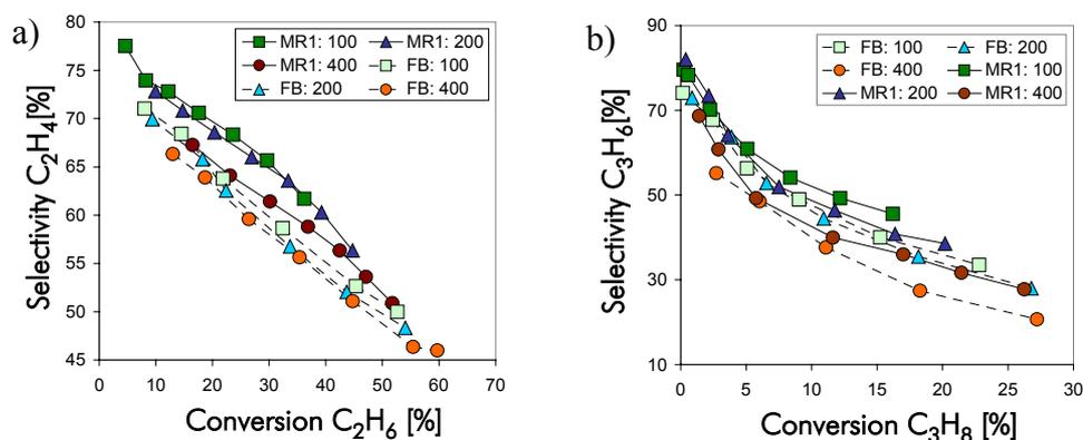
Figure 1: a) selectivity ethylene vs. conversion, b) selectivity propylene vs. conversion:  $C_2H_6^{in} = 1,5\%$ ,  $C_3H_8^{in} = 1\%$ ,  $O_2/C_nH_m = 1$ , WHSV = 100-400kgs/m<sup>3</sup>, catalyst:  $VO_x/\gamma-Al_2O_3$ , (V: 1.4%), BET: 157m<sup>2</sup>/g, particle:  $d_p = 1.0$  mm
