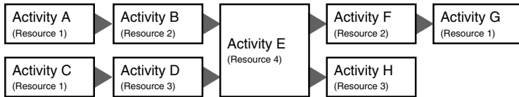
Figure 3.2. Sequence definition for a generalized job type (precedence network).
