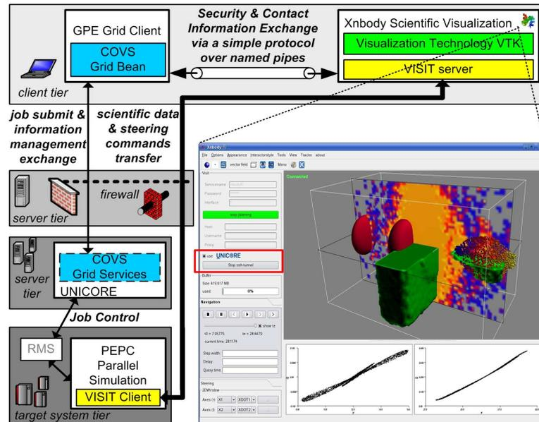
Figure 3: Xnbody uses the 'use UNICORE' checkbox to seamlessly connect to supercomputing sites via security information based on UNICORE.
