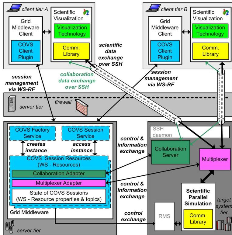
Figure 1: COVS architecture for UNICORE, gLite or Globus Toolkits as Grid middleware. Web services are used for communication as well as SSH tunnels for the bi-directional transfer of scientific data and steering commands.
