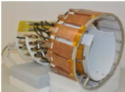
Fig. 3: The complete RF setup with the Tx array, Rx array and the preamplifier assembly
