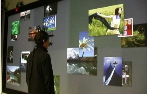
Figure 6: GazePic demo. The user can move the images by using his/her gaze.
