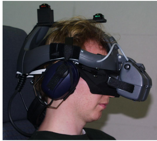
Figure 1: Left: 180^\circ \times 50^\circ FOV half-cylindrical projection screen. Right: Subject wearing HMD, FOV 40^\circ \times 30^\circ .
