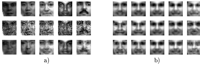
Figure 6.2: a) Denoising performance on 5 face images of the testing set. The original images are on the first row, the noisy images on the second row, and the predicted noise-free images on the third row. b) Illustration of three output feature vectors \mathbf{v}_i in \mathbf{V} , one in each row (in a nutshell, the feature vectors span the subspace of the output relevant to the regression process). The significance of these features is shown by perturbing a particular image in the direction parameterised by each of the vectors. The middle column corresponds to the mean image over all faces in the training set, while to the left and right we add \alpha \mathbf{v}_i for a small \alpha . The columns correspond respectively to \alpha \in [-0.2, -0.1, 0, 0.1, 0.2] .
