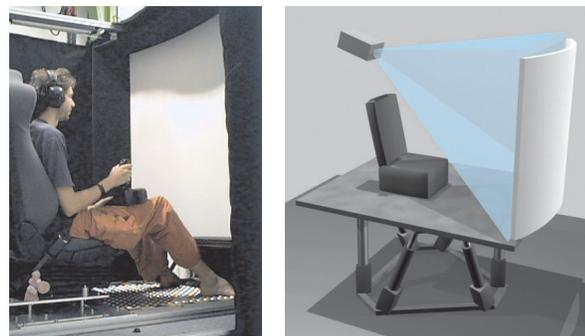
Figure 1: Motion platform and projection screen ( $86^\circ \times 63^\circ$ )
