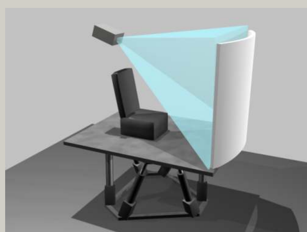
Fig. 5: Schematic experimental setup showing the 6 degree of freedom motion platform and the projection setup.
