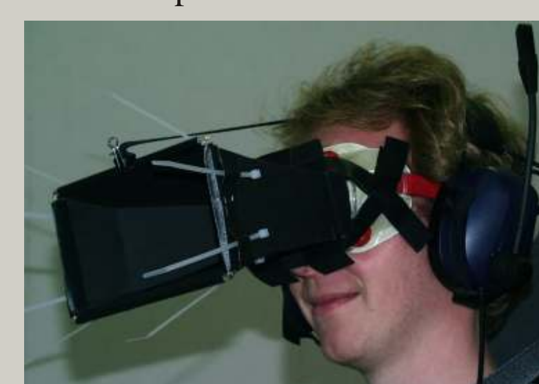
Fig. 3: Participant wearing blinders (vision delimiting cardboard goggles) and headphones reducing the FOV to that of the HMD (40°x30°).
