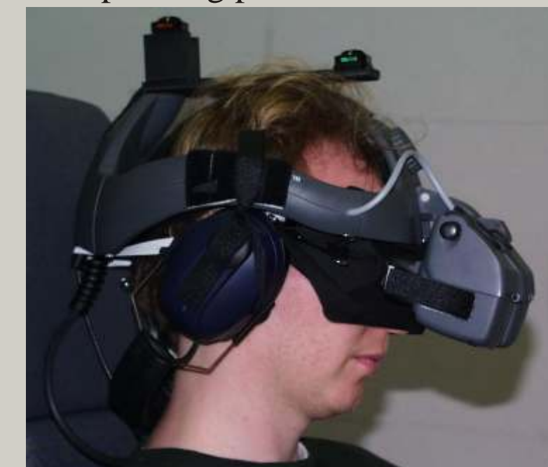
Fig. 2: Participant wearing position-tracked head-mounted display (40°x30° FOV, 1024x768 pixel) and active noise cancellation headphones.
