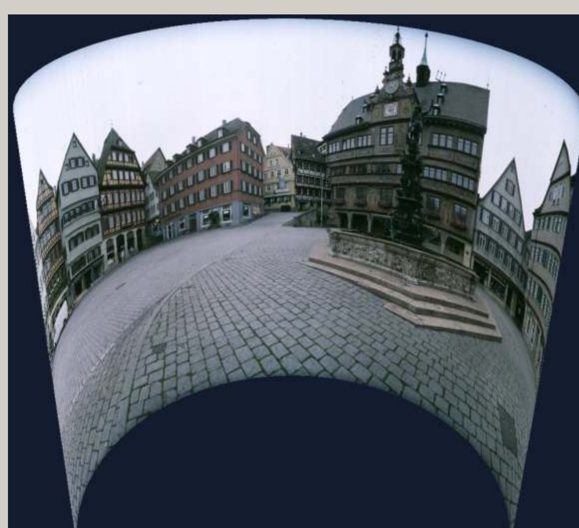
Fig. 6: The model was created by wrapping a 360° round shot photograph of the Tübingen market place (see Figure below) onto a cylinder. This creates an undistorted view for the observer positioned in the center of the cylinder.
