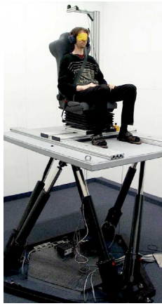
Figure 1: The Stewart-Platform motion simulator. The subject is seated blindfolded and with headphones on the platform. The platform is able to move in all 6DOFs independently.
