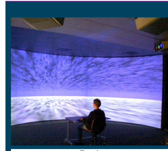
Figure 1: Experimental setup with the half-cylindrical projection screen displaying optic flow from the 3D field of blobs.
