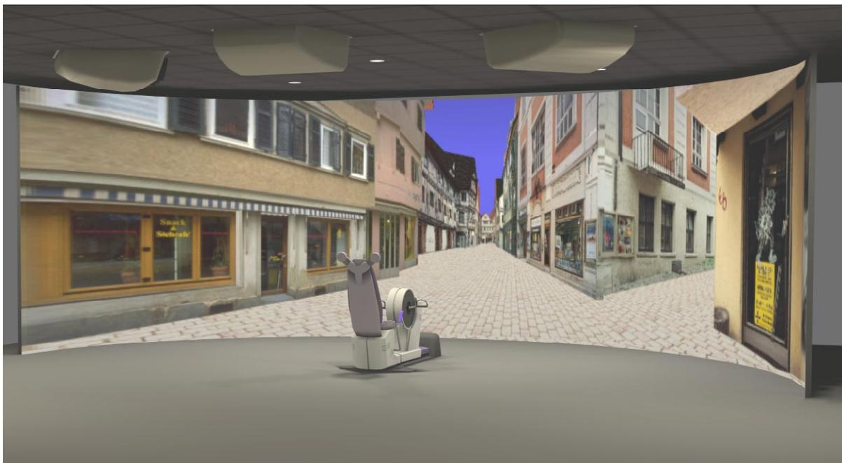
**Figure 3.** VRbike in front of the large screen projection screen. The panoramic image of virtual Tübingen is projected by three ceiling mounted CRT projectors in such a way that at the head position of the cyclist a realistic 180 degree view of Tübingen can be experienced while cycling through the model
