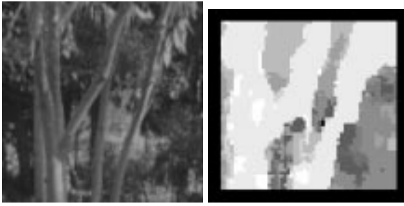
Figure 15: Depth from motion parallax, using image zoomed by a factor of 2. Camera is translating left, with the resulting optical flow and grey-level shaded relative depth map. Lighter areas indicate objects closer to the camera.
