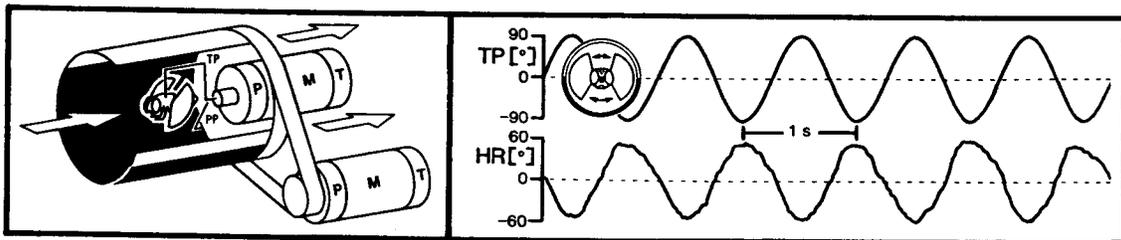
**Figure 1:** Compensatory head roll (HR) of *Calliphora* elicited by imposed sinusoidal roll of the fly (TP, 1Hz,  $\pm 90^\circ$ ) during tethered flight. Video recordings were made through the entrance nozzle of the suction wind tunnel.
