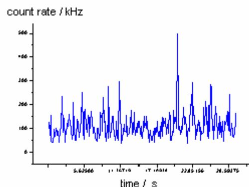
Figure 1: Fluorescence count rate of a 0.2nM solution of quantum dots excited with 820 nm (average laser power 7.5 mW, emission < 700 nm).
