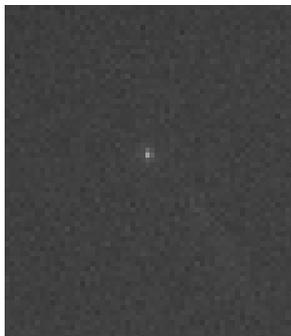
Figure 12: Image of a single enlarged quantum dot representing the Point Spread Function (PSF) of the microscope.
