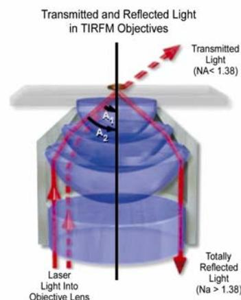
Figure 6: Radiation pathway within an objective-type TIRF-microscope
