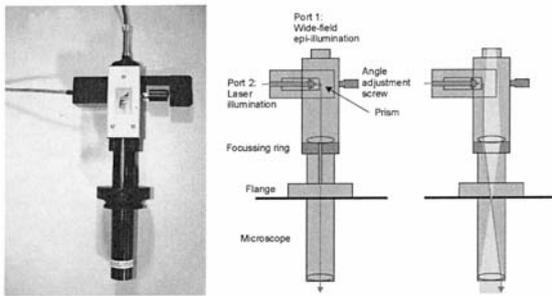
Figure 7: TILL-TIRF dual port epifluorescence condenser
