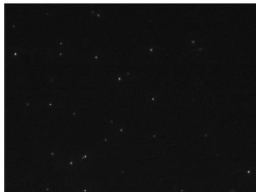
Figure 10a+b: Improved imaging conditions of the TIRF-microscope mode as compared to conventional bright field illumination using fluorescent beads of about 100 nm diameter.
