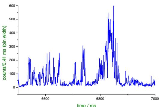
Figure 3: Multichannel scaler (MCS) trace of a 0.2 nM solution of QDs (bin width 0.41 ms).
