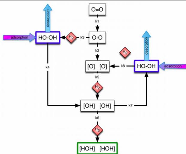
**Scheme 1.** Reaction network of the direct H<sub>2</sub>O<sub>2</sub> synthesis: direct formation of H<sub>2</sub>O<sub>2</sub> (a) and H<sub>2</sub>O (b), and decomposition of H<sub>2</sub>O<sub>2</sub> to H<sub>2</sub>O (c).
