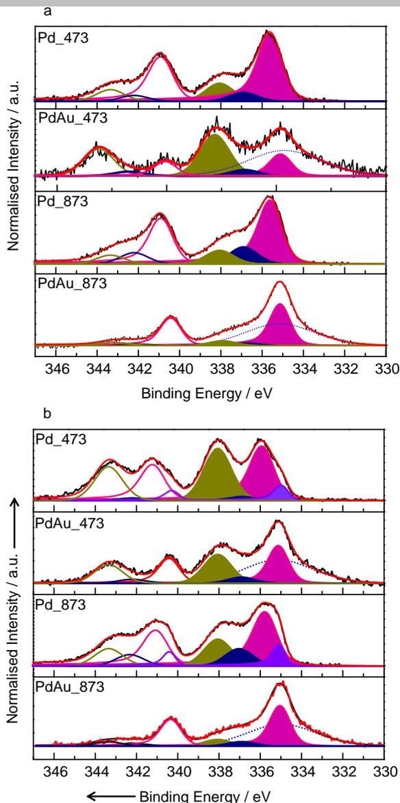
**Figure 7.** Pd3d XP core level spectra for the samples fresh (A) and after 12 minutes of reaction (B) at KE 600 eV. Fitting: Pd(0) (violet peak); Pd(I) (magenta peak); Pd(II) (blue peak); Pd(III) (ocher yellow peak); dashed line in PdAu873 and PdAu473 is the Au3d<sup>5/2</sup> peak.
