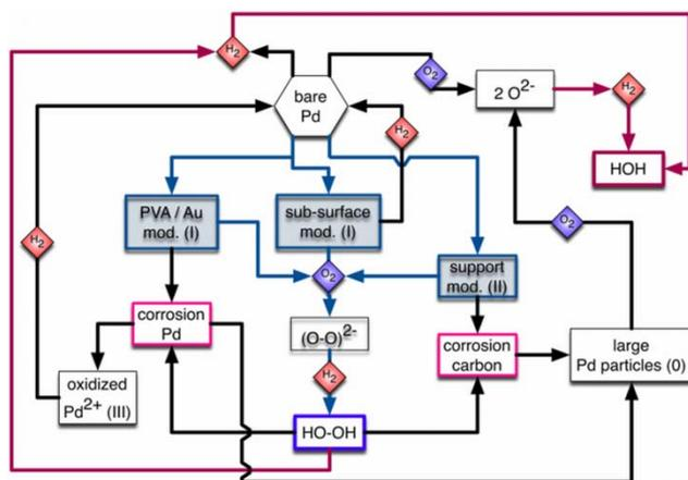
**Scheme 2.** Reaction system of H<sub>2</sub>O<sub>2</sub> synthesis. The numbers in brackets refer to the XPS assignments discussed. The blue arrows designate the desired selective reaction path, the red arrows indicate the unselective deep hydrogenation and the black arrows refer to the structural deactivation pathways of the catalyst.
