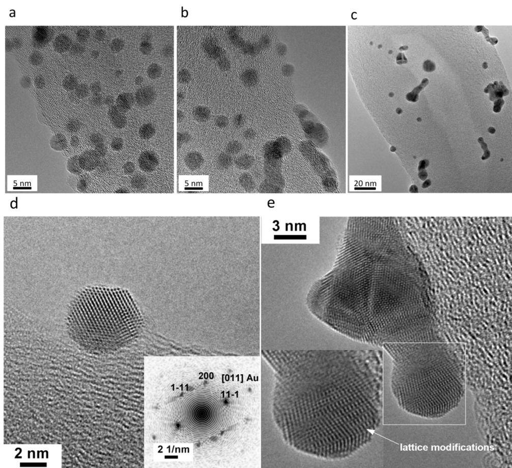
Figure 4. TEM on PdAu<sub>873</sub> (A); PdAu<sub>873u</sub> (B) PdAu<sub>873u</sub> after 3h reaction; HRTEM on nanoparticles on PdAu<sub>873</sub> (D); HRTEM on sintered nanoparticles on PdAu<sub>873u</sub> after 3h reaction (E).
