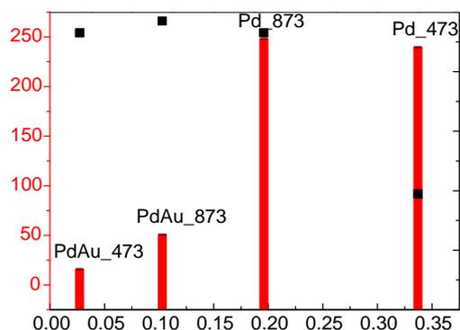
**Figure 2.** H<sub>2</sub>O<sub>2</sub> cumulative production (molKg<sup>-1</sup>h<sup>-1</sup>) and selectivity at 20 min vs specific Pd surface area (m<sup>2</sup>g<sup>-1</sup>) as determined by CO chemisorption.
