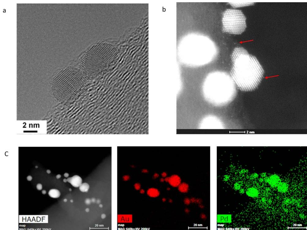
Figure 3 HRTEM on PdAu<sub>473</sub> (A) and HAADF-STEM (B), EDX mapping (C).
