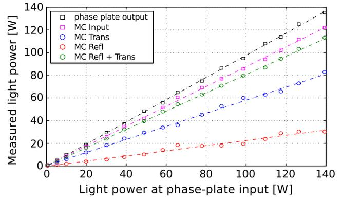
FIG. 4 (color online). Measurement of the light power at different locations in the setup as a function of the injected laser power. Statistical uncertainties in the measurement data are smaller than the marker’s size and here not reported. Systematic errors in the calibration of each power curve are of order 5%.
