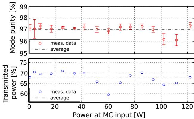
FIG. 6 (color online). Top:  $LG_{33}$  purity of the beam transmitted by the mode cleaner. Bottom: fraction of the injected light power which is transmitted from the resonant mode cleaner (circles). Dashed lines show average values. Statistical errors are negligible, while calibration uncertainty is here of order 7%.
