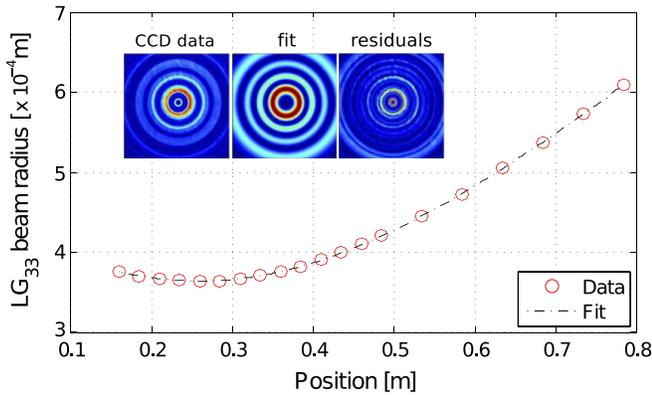
FIG. 2 (color online). Profile of the  $LG_{33}$  beam injected into the MC cavity, with best fit shown for comparison. The insets show an example of fitting of a  $LG_{33}$  beam, with the intensity patterns of a measured beam compared to the fit and related residuals.
