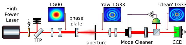
FIG. 1 (color online). Cartoon of the experimental setup described in the Letter. The main components are labeled. Beam dumps, steering mirrors, wave plates, and polarizers are not shown.
