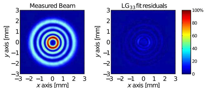
FIG. 5 (color online). Intensity profile of the 83 W  $LG_{33}$  beam transmitted by the MC cavity (left) compared with fit residuals (right). Maps have same units and scale.
