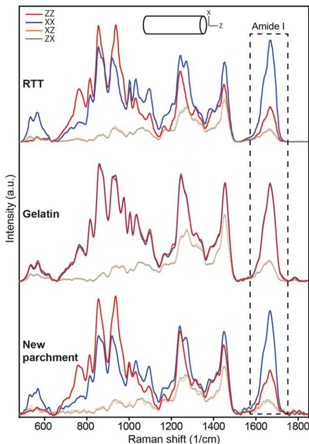
**Fig. 2** Polarized Raman spectra of rat tail tendon fiber (top), gelatin (middle) and newly prepared parchment fiber (bottom). The dashed box highlights the amide I region used for evaluating orientation parameters. Amide I anisotropy is evident [comparing XX (blue) and ZZ (red) configurations] for RTT and new parchment fibers, but completely vanishes for the gelatin sample.
