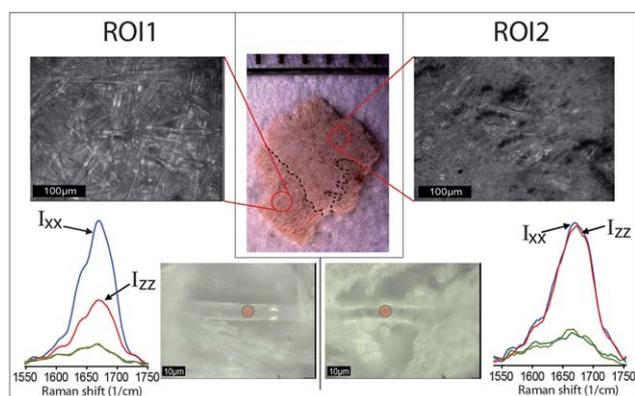
**Fig. 3** Stereo- and optical microscopy images (top) of two ROIs of the Temple Scroll fragment examined in this study. Collagen fibers can be found in both ROIs. The bottom part shows single collagen fibers in both ROIs and polarized Raman spectra in the amide I region performed on the fibers in correspondence of red spots. A clear difference in anisotropic behavior can be observed.
