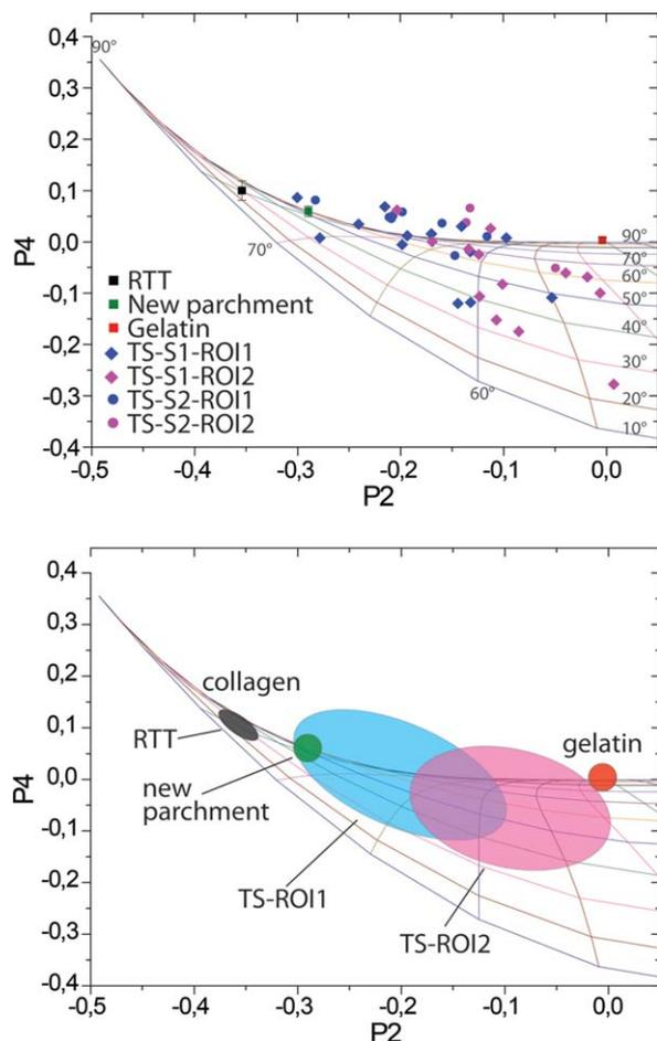
**Fig. 4** Top:  $P2$ – $P4$  plot of orientation parameters relative to all samples analyzed in this study. Bottom: characteristic regions found for different samples indicative of different states of preservation of collagen.
