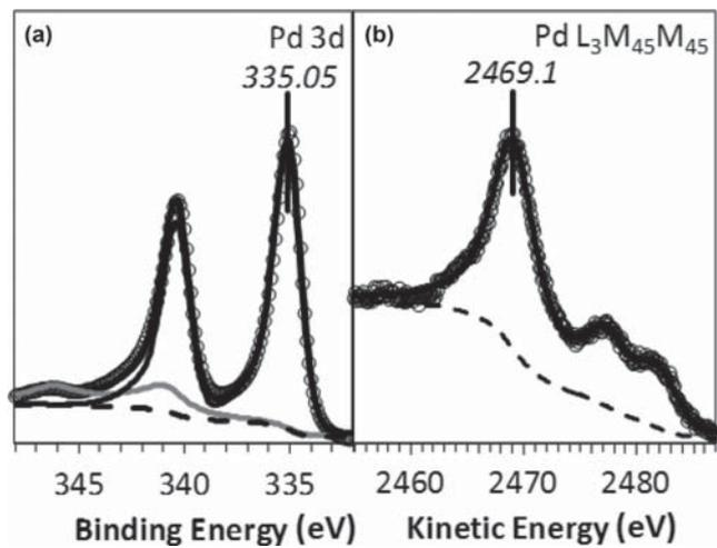
FIG. 4. (a)  $3d$  XPS and (b)  $L_3M_{45}M_{45}$  Auger spectra from freshly cleaned Pd(111).
