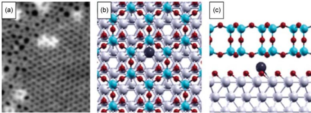
FIG. 2. (Color online) (a) STM image of  $\sim 5 \times 10^{12}$  Pd/cm<sup>2</sup> on bilayer SiO<sub>2</sub>/Ru(0001) at  $\sim 5$  K. Image is  $10 \times 8.4$  nm<sup>2</sup>, and was taken at constant current, with  $V_s = 2$  V and  $I_T = 100$  pA. (b) Top and (c) side views of a Pd atom bound at the interface between the bilayer SiO<sub>2</sub> film and the O-covered Ru(0001) substrate. Blue, red, light gray, and dark gray spheres represent Si, O, Ru, and Pd atoms, respectively.
