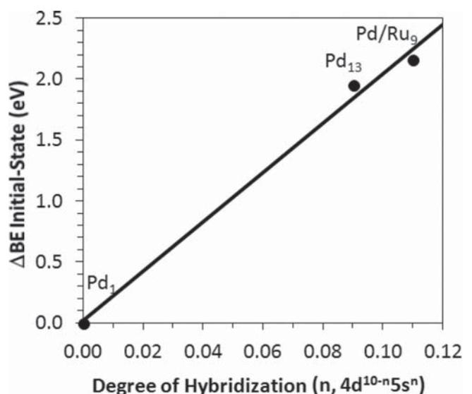
FIG. 6. Initial-state shifts (vs Pd<sub>1</sub>) to the Pd  $3d$  BEs are plotted relative to the degree of  $4d$ - $5sp$  hybridization for the Pd<sub>1</sub>, Pd<sub>13</sub>, and Pd/Ru<sub>9</sub> clusters depicted in Fig. 1.
