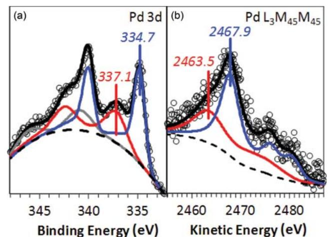
FIG. 3. (Color online) (a) 3*d* XPS and (b) *L*<sub>3</sub>*M*<sub>45</sub>*M*<sub>45</sub> Auger spectra from  $\sim 9 \times 10^{13}$  Pd/cm<sup>2</sup> on bilayer SiO<sub>2</sub>/Ru(0001) at  $\sim 150$  K.
