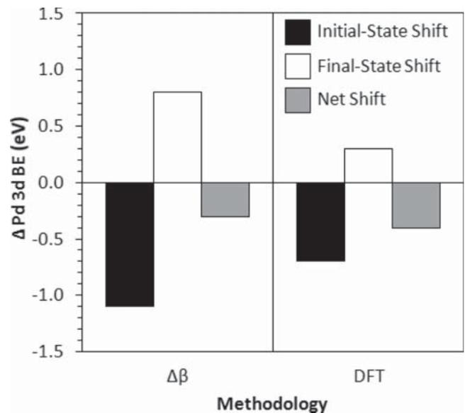
FIG. 5. Experimentally measured changes to the  $3d$  BE of the SCS-like Pd ( $\Delta\beta$ ), relative to bulk, are compared to those derived from theoretical calculations (DFT) of the  $\text{SiO}_2$ /Ru-supported system described by Fig. 2. Included with the total expected/detected shifts (gray) are the partitioned contributions attributed to changes in the initial- (black) and final-state (white) configurations of the photoemission process.
