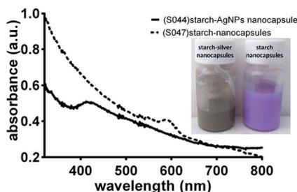
Fig. 2 UV-visible spectra of starch-silver nanocapsules versus starch only nanocapsules; the inset shows the appearance of the mini-emulsion solutions.
