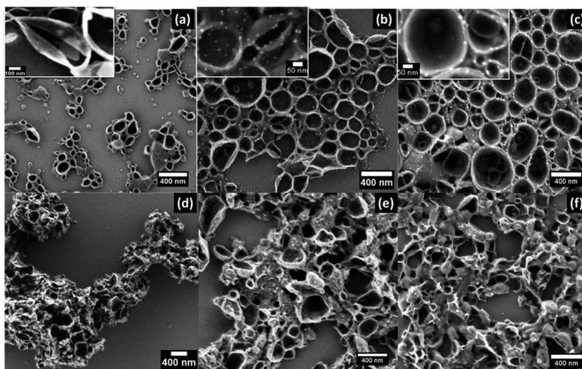
Fig. 3 SEM images of starch nanocapsules with and without silver nanoparticles: (a) S043, (b) S044, and (c) S045 which were synthesized with  $\text{AgNO}_3$  and (d) S046, (e) S047, and (f) S048 which were synthesized without  $\text{AgNO}_3$ .
