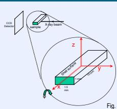
Fig. 4: Sample geometry
