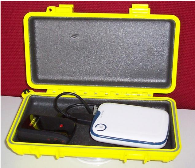
**Fig. 3.2.1** Qstarz BT-Q1000XT GPS logger (left) and Mobile Power Pack VT-PP-320b (right). Both were packed in a waterproof OtterBox 3000.
