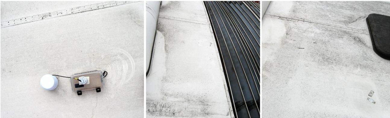
**Fig. 3.4.2** Roof pictures of **bus 2** from front to back. The center position shows black dirt and dark elastic lamella, both lowering the albedo. The back position has a black emergency exit hatch.
