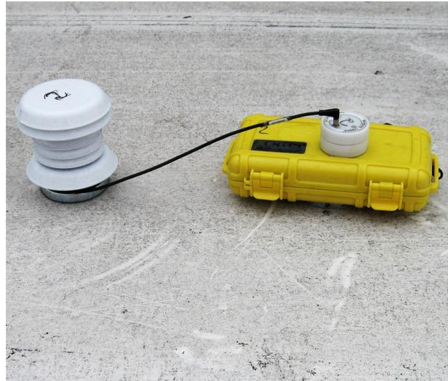
**Fig. 3.2.2** The instrumentation on the bus roof. The logger is glued on the OtterBox and could easily be turned up in order to read the data via USB cable.
