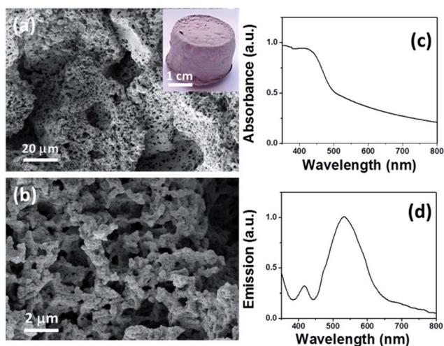
Fig. 1 (a and b) SEM images of B-(Boc-CB)<sub>2</sub>-BO, the inset is a photograph of the monolithic polymer, (c) DRS UV/Vis, and (d) photoluminescence spectra.
