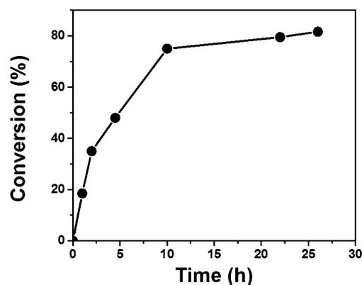
Fig. 2 Photopolymerization of methyl methacrylate using B-(Boc-CB)<sub>2</sub>-BO as a heterogeneous photoinitiator at room temperature under visible light.
