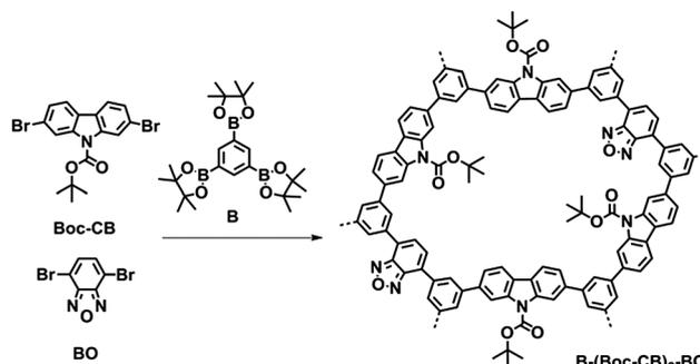
Scheme 1 Synthesis route to B-(Boc-CB)<sub>2</sub>-BO using palladium catalyzed Suzuki–Miyaura cross-coupling reaction via high internal phase emulsion (HIPE) polymerization and its idealized structure. Reaction conditions: Pd(PPh<sub>3</sub>)<sub>4</sub>, K<sub>2</sub>CO<sub>3</sub>, Span® 80, H<sub>2</sub>O–toluene, 80 °C, 12 h.
