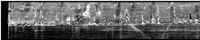
Fig. 7. Example of a large propagated crack in CFC at the interface tile – heat sink.
