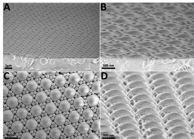
Fig. 4 Binary monolayer of PS colloids with a diameter of 1  $\mu$ m and 225 nm embedded in a film of PBCA (A and B). Micrographs (A) and (B) reflect the situation at the air–water interface. Micrographs (C) and (D) show monolayers of the same colloid mixture after deposition on solid substrates.
