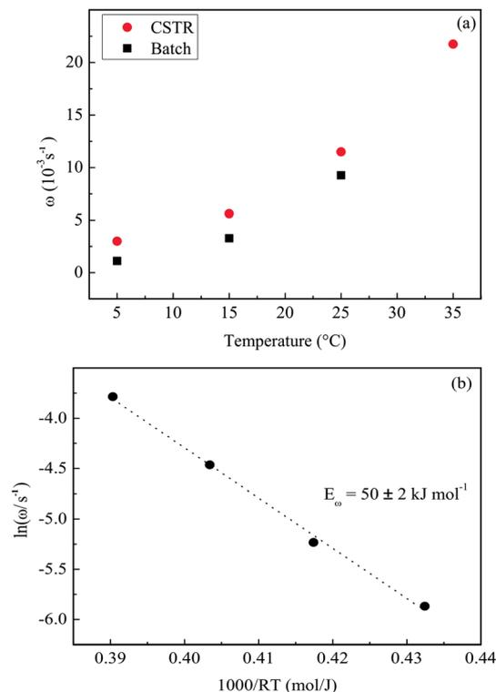
Fig. 7 (a) The effect of temperature on the oscillatory frequency  $\omega$ , for the bromate–oxalic acid–acetone–cerium system operated in batch and also in a CSTR. (b) Arrhenius plots using the oscillatory frequency,  $\omega$ , for the system operated in a CSTR. Data for experiments in batch as in Fig. 1 and for the open system as in Fig. 6.
