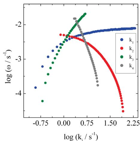
Fig. 10 Influence of each  $k_i$  on the oscillatory frequency for the CSTR version of the Brusselator model, set ODE (3) with  $k_f = 0.10 \text{ s}^{-1}$ . Each rate constant was varied individually while the others would obey the following set  $\{1, 2, 1, 2\}$ .  $A_0 = B_0 = 20$ .
