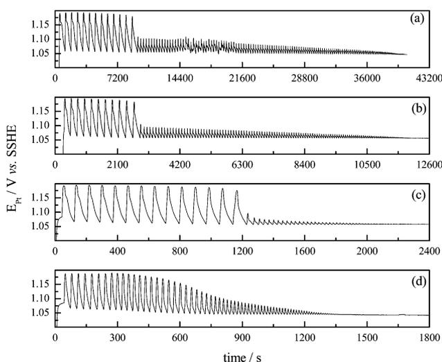
**Fig. 2** Time-series of the platinum electrode for the bromate–oxalic acid–acetone–cerium oscillatory system operated in batch at (a) 5, (b) 15, (c) 25 and (d) 35 °C. Initial concentrations:  $[\text{H}_2\text{SO}_4]_0 = 1.42 \text{ mol L}^{-1}$ ;  $[\text{NaBrO}_3]_0 = 0.010 \text{ mol L}^{-1}$ ;  $[(\text{COOH})_2]_0 = 0.025 \text{ mol L}^{-1}$ ;  $[\text{CH}_3\text{COCH}_3]_0 = 0.157 \text{ mol L}^{-1}$  and  $[\text{Ce}_2(\text{SO}_4)_3]_0 = 0.0005 \text{ mol L}^{-1}$ .
