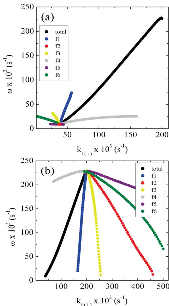
Fig. 9 The curve in black shows how oscillatory frequency depends on the flow rate for the CSTR version of the Brusselator model using the  $\{1, 2, 1, 2\}$  rate constants set. The colorful lines indicate the dependency of the oscillatory frequency on the individual rate constants  $k_{f,i}$  found in the set ODE (4), at low and high flow values,  $k_0 = 40$  in (a), and  $k_0 = 200$  in (b).  $A_0 = B_0 = 20$ .
