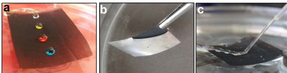
Figure 2. Superamphiphobic meshes floating on liquid. (a) Drops ( 5 \mu\text{L} ) of DMF (white), peanut oil (yellow), n -hexadecane (red), and water (blue) deposited onto the superamphiphobic mesh floating on n -hexadecane. For better visualization, the drops and the n -hexadecane subphase were dyed with oil red O; (b) A superamphiphobic mesh is pushed into n -hexadecane; (c) Water drops jetted on a superamphiphobic mesh floating on water.
