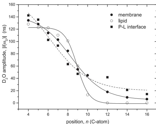
FIGURE 2 Dependence of  $D_2O$ -ESEEM amplitudes on position,  $n$ , in the chain of ionized spin-labeled stearic acid ( $n$ -SASL) at pH 8.9: in Na,K-ATPase membranes (solid circles,  $I_m$ ) and in bilayer membranes of the extracted lipids (open circles,  $I_f$ ). Solid squares are the  $D_2O$ -amplitudes at the protein-lipid interface,  $I_b$ , that are calculated from the membrane and lipid data according to Eq. 4. Lines are fits of a Boltzmann sigmoidal profile according to Eq. 3.
