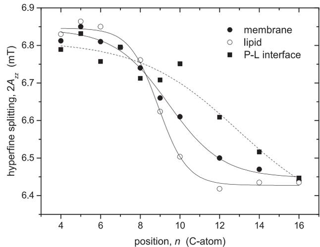
FIGURE 4 Dependence of the outer hyperfine splitting,  $2A_{zz}$ , on position,  $n$ , in the chain of ionized spin-labeled stearic acid ( $n$ -SASL) at pH 8.9: in Na,K-ATPase membranes (solid circles) and in bilayer membranes of the extracted lipids (open circles). Solid squares are the outer hyperfine splittings at the protein-lipid interface that are calculated from the membrane and lipid data according to Eq. 5. Lines are fits of a Boltzmann sigmoidal profile according to Eq. 3.
