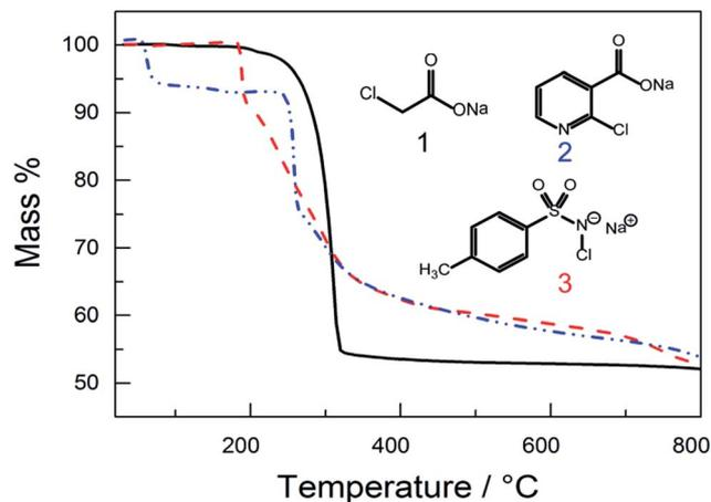
Fig. 1 TGA curves, recorded with  $10 \text{ K min}^{-1}$  under a flow of  $\text{N}_2$ , track the thermal decomposition of sodium-2-monochloroacetate (1 NaAc-Cl), sodium-2-chloropyridine-3-carboxylate (2 NaPyr-Cl) and *N*-chloro-*p*-toluenesulfonamide sodium salt (3 CT).
