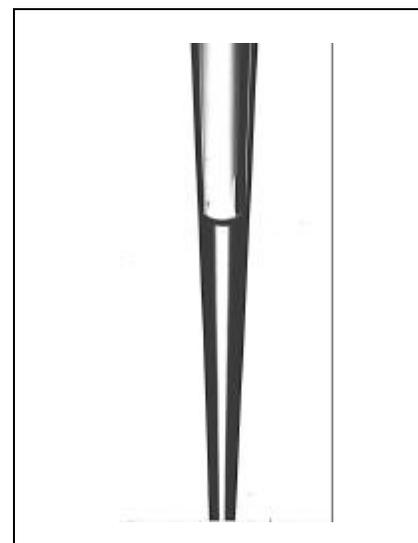
Figure 2. A smooth interface free from air bubbles results when LIX is drawn into a microelectrode previously filled with electrolyte.
