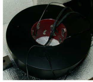
Figure 3: Heating mats at the inner boundary \Gamma_1 attached by magnets.
