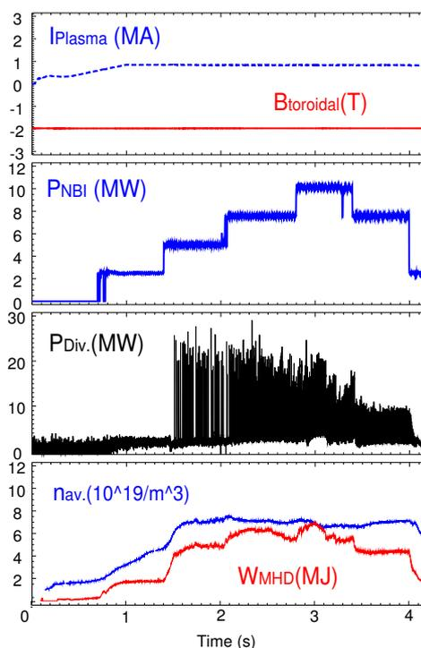
**Figure 2:** Temporal evolution of some discharge parameters in the Upper Single Null (USN) discharge (#16724) in ASDEX Upgrade.
