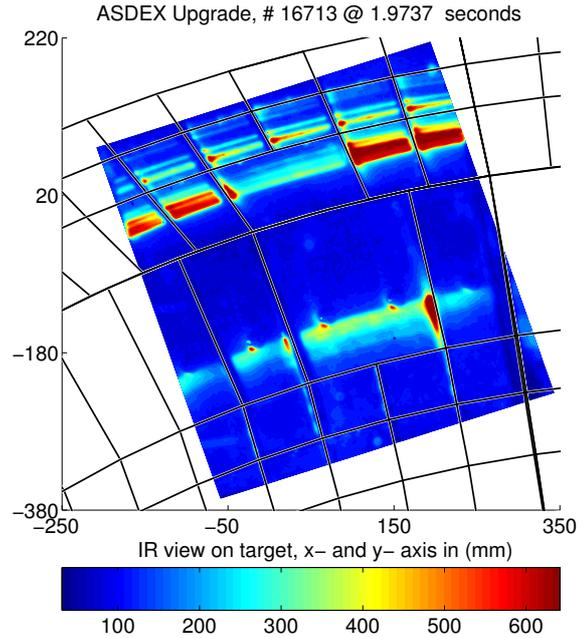
**Figure 3:** The power deposition pattern during this type-I ELM event shows a characteristic non-axisymmetric structures most prominent in the remote area of the outboard strike line (# 16713). Temperature in  $^{\circ}C$
