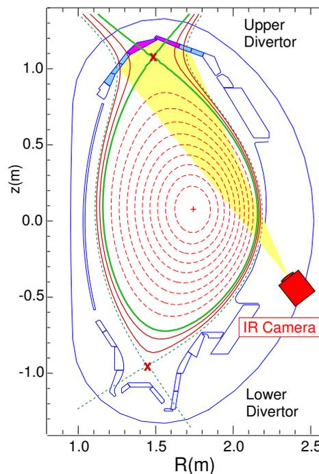
Figure 1: *Poloidal cross section of ASDEX Upgrade with Upper Single Null magnetic equilibrium configuration (#16724).*
